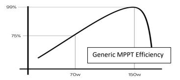
Below and example of an all-round MPPT controller efficiency. Not reaching that very peak of 99% efficiency but instead working at a very high efficiency no matter what solar panel, what weather or sun angle we experience.
